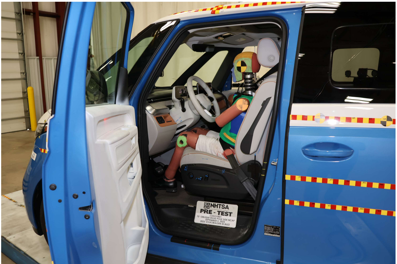
Photo No. 023 - Pre-Test Left Side View of Dummy Showing Belt and Chalking
