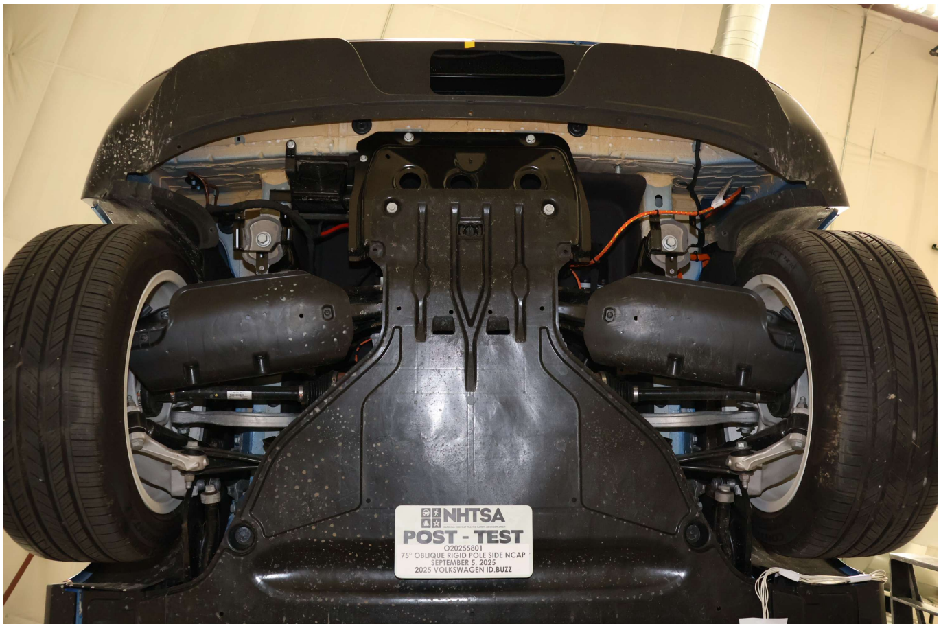
Photo No. 305-17 - Post-Impact View of Electric Propulsion Drive
